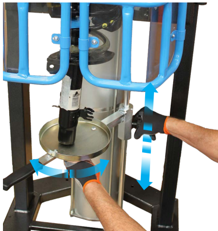
STEM SUPPORT ADJUSTABLE IN HEIGHT AND 180° ADJUSTABLE
