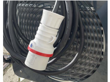
ELECTRICAL CABLE WITH 4-POLE PLUG
