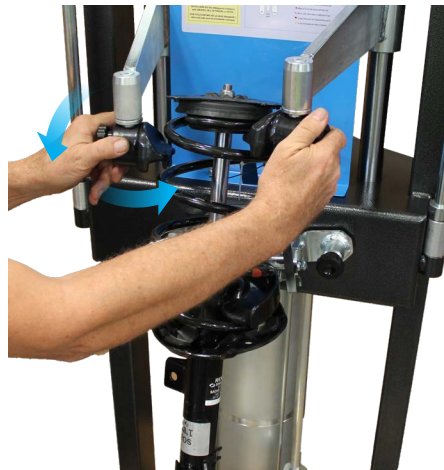
UPPER FLOATING CLAMPS , these floating clamps allow a better grip on the spring, dynamically adapting during the different compression phases.
