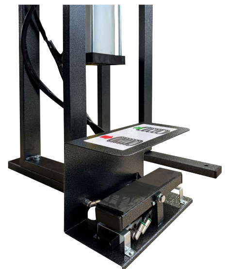
THE FOOT-PEDAL WORKS ONLY WHEN THE SAFETY VALVE IS CLOSED; IF IT IS OPEN THE FOOT-PEDAL IS BLOCKED
